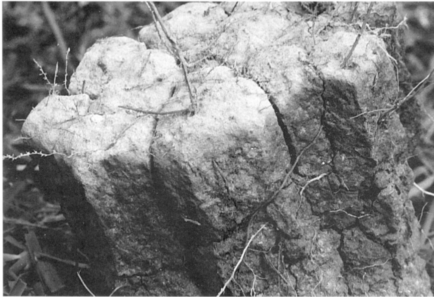
A cluster of strong medium columnar peds. The cluster is about 135 mm across.
