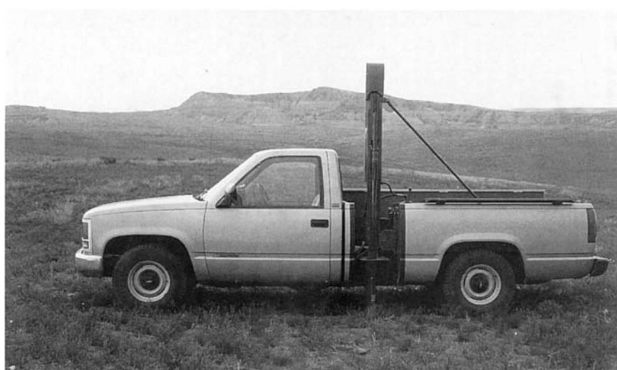
A hydraulically mounted sampling tube mounted on a pickup truck. The open-faced tube is in place. Hydraulic controls are at the right.
